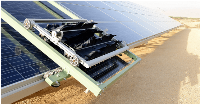
Figure 9: Ecoppia E4 Water-free automated cleaner
